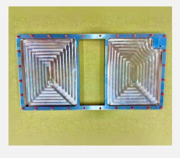
Our in-house precision masking department enables us to provide comprehensive turnkey solutions. Painted or coated precision machined components demand meticulous masking, as they frequently feature intricate and delicate details that must be protected from the coating application.
